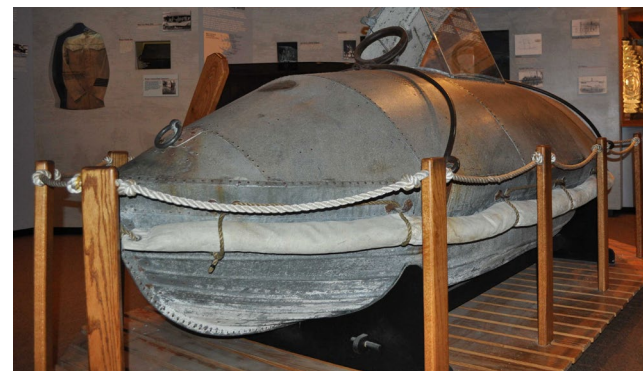
The metal life car was used to pull at least five or six adults from the shipwreck to the beach. NC Maritime Museum.
