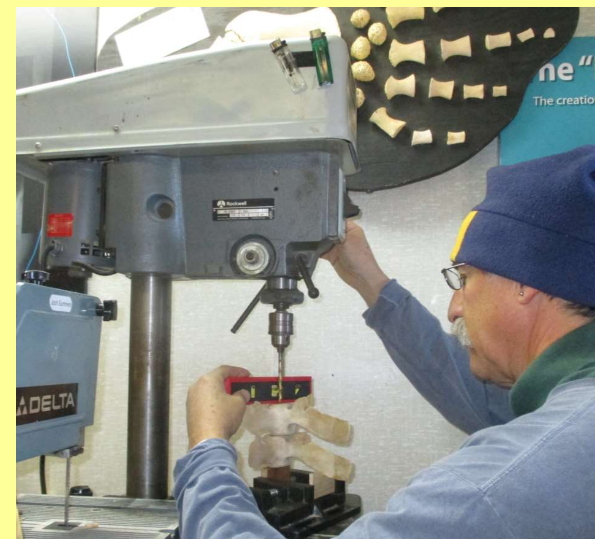
Fig. 10. Using a drill press, vice, torpedo level, and the previously drilled adjacent vertebra assured proper alignment of the spine on the 1/4" steel rod.
