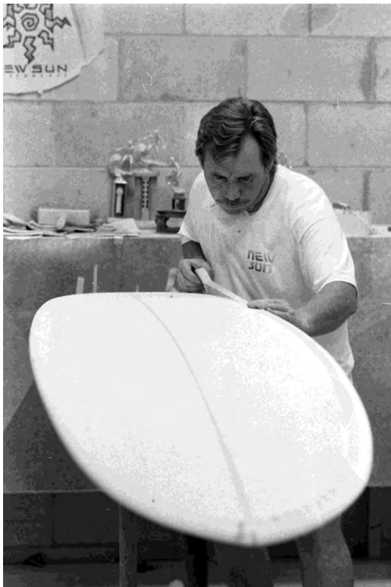
Surfboard shaping parallels some of the early methods of boatbuilding in a way. There are a few measurements and a lot of examining by the eye. If it doesn't look right the shaper sands a little more here or a little more there. Mickey McCarthy working on one of his New Sun surfboards in Dare County, 1990. Image courtesy of The Outer Banks History Center, Manteo, NC, Drew C. Wilson Collection.
