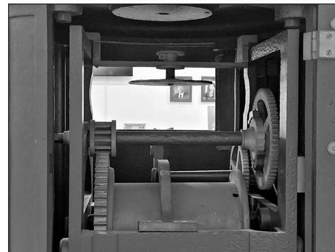
Clockwork mechanisms from the 1854 Fresnel lens.
